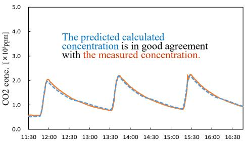
The coefficient of determination COD of reliability evaluation index is 0.926
