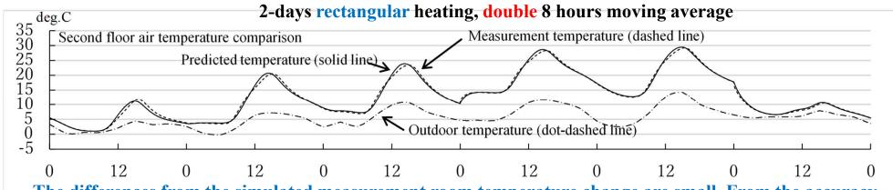
The differences from the simulated measurement room temperature change are small. From the accuracy comparison of U values in the previous slide, we can conclude that the system identification accuracy is improved by double moving average even with the square waveform heating.
